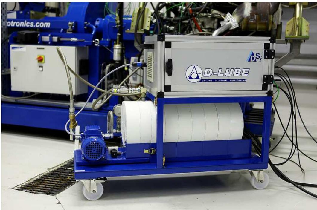
**FIG 2: D-LUBE EQUIPMENT INSTALLED IN A TEST CELL FOR REAL-TIME FUEL DILUTION MEASUREMENT ON AN I.C. ENGINE**
