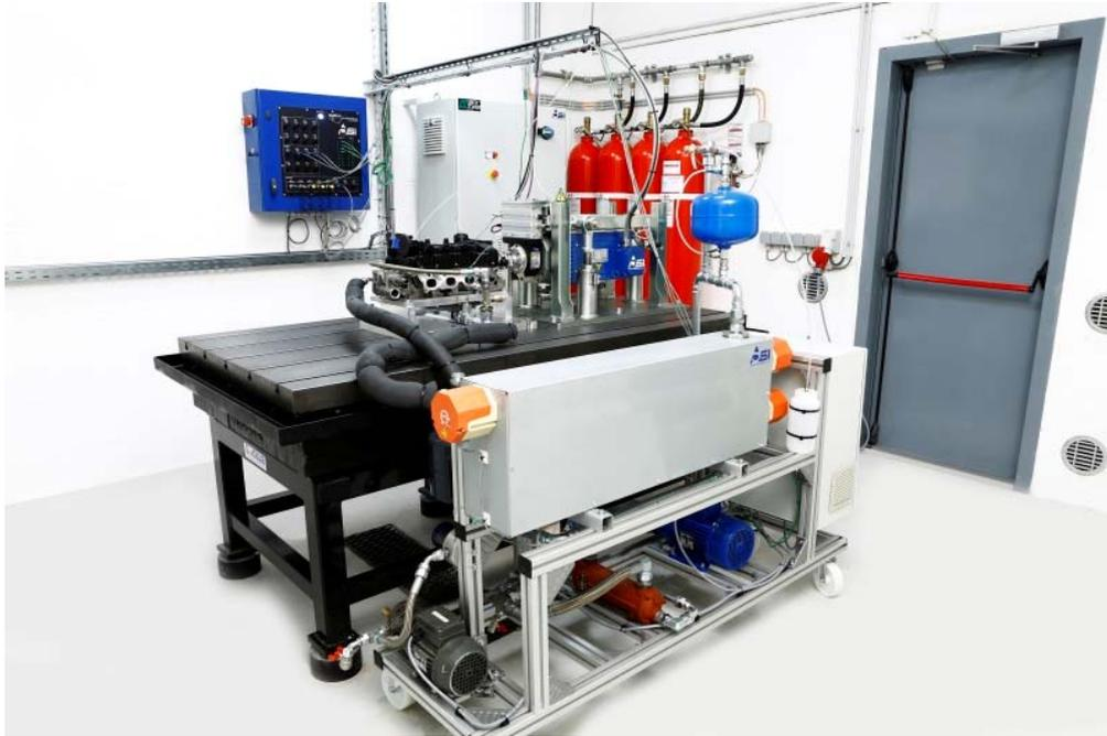
New test rig dedicated to the study of friction, lubrication and wear on valvetrain
