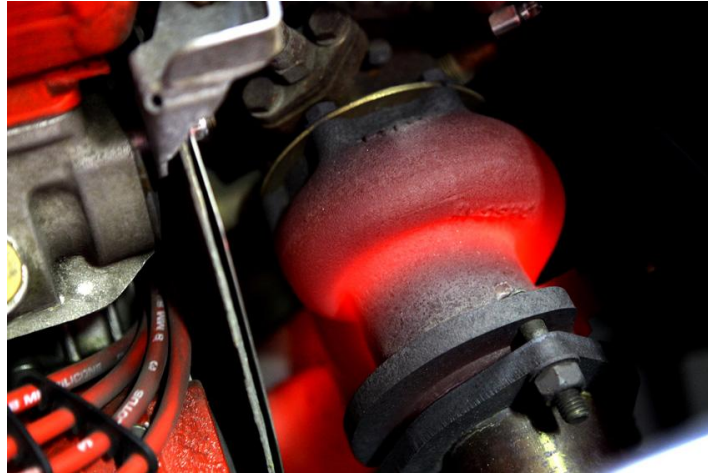
OIL CONSUMPTION FROM BOTH STAGES OF A TURBOCHARGER ARE MONITORED INDEPENDENTLY
